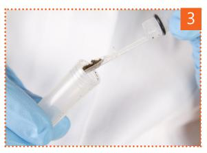
■ Dilute its content in the liquid of the small tube called sample
