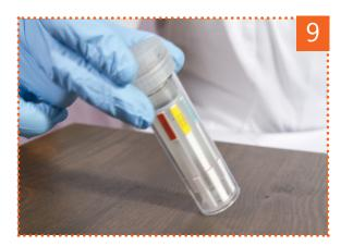
Sometimes, especially when the sample isn't homogenized, liquid migration can stop on one or more strips. In that case, tap the end of the strip tube on hard surface to allow migration to start again.
